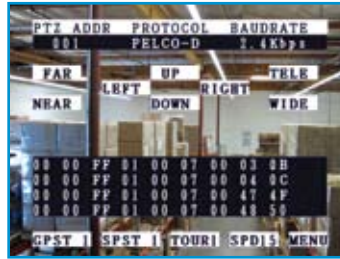
PTZ protocol analyzer can be used in-line to troubleshoot keyboard controllers and cameras
