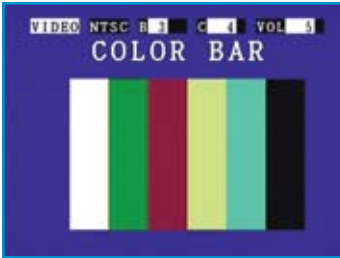
Test pattern generator outputs color bar and solid red, green, and blue screens in NTSC or PAL format
