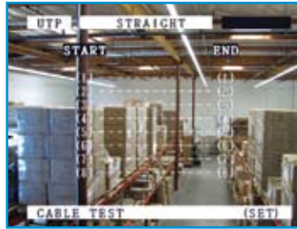
Wire map tester for UTP cabling with clear display of fault condition
