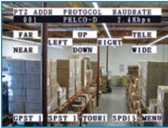
PTZ control with addressing for up to 255 cameras, 20+ protocols and 4 baud rates with selectable RS422/488 communications
